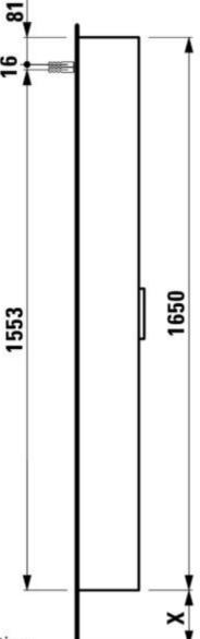
( = The exact hight must be set during installation.
