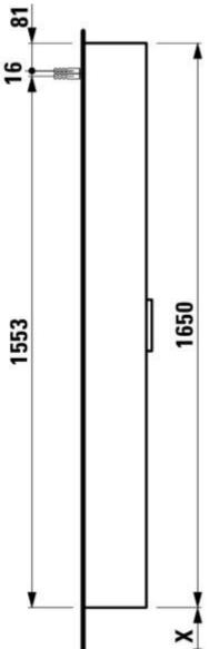
X =The exact hight must be set during installation.
